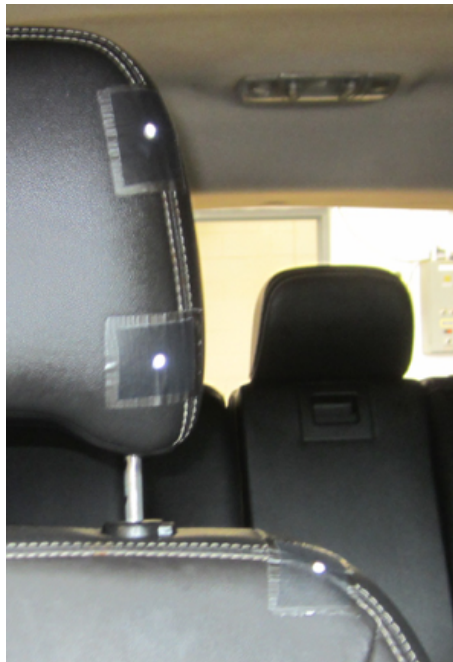
Reflective markers placed on seats
