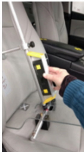
Record seat back and seat cushion angles
