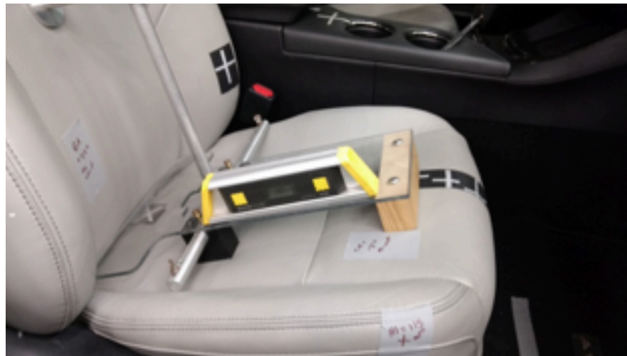
Record seat back and seat cushion angles
